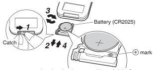
Load so that battery + side and side of battery tray with + mark face same direction
