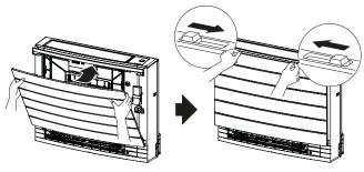
3 Push on the sides of the front panel to make sure the front panel is securely fixed.
