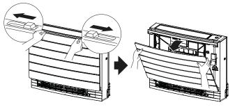
2 Open the front panel and undo the string.
