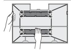
2 Insert the filter tabs to the claws on the bottom (d). Hold the air filter by the filter knob (b) and insert the air filter tab to the claw (c) on the top. Insert the air filter tabs to the claws (a) on the sides. Make sure the air filter is securely fixed in all positions.
