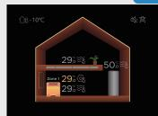
Select the target device, and press and to adjust the set temperature. Set temperature adjustment is possible regardless of the device status.
