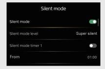
There are two timers. When there is no active timer, the unit operates completely in Silent mode or Boost mode. If a timer is active, the unit operates in Silent mode or Boost mode only when the timer is active. You can also set the level of Silent mode or Boost mode in Mode setting. (Boost mode is only available for specific units.)
