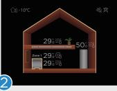
Press or to select a device. A selected device is highlighted (the surrounding lights up).
