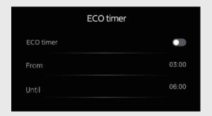
You can see "ECO timer" on the bottom of the page. You can set the start time and end time of the timer and activate the timer. If the timer is active, the unit will run the ECO curve only during the time period set on the timer. If the timer is deactivated, the unit will constantly run the ECO curve.
