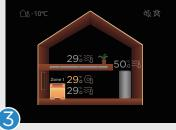
Press . The color of the device turns bright orange or bright blue (depending on which operation mode you select), which means the heat pump is now Heating or Cooling for that area.
