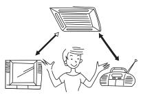
Put the TV or radio away from the air conditioner at least 1 meter, or signal will be interfered.
