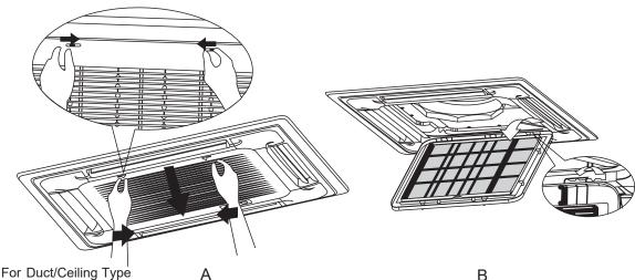
Push the grill switches to the arrow directions, then open the air-in grill downwards. Turn back the air filter fixing block, then take out the air-in grill.
